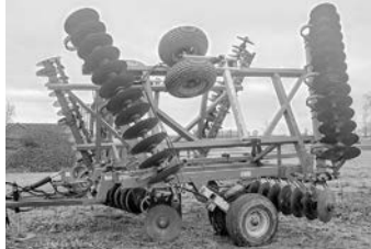
'01 Krause 4991-31 WR rock flex 31' disc, 9" blade space, 21.5" blades, hyd. leveling, rear hitch, hyd. hose hook up, $13,500
